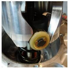
The "X" on the helix is aligned with the x on the clutch.
