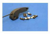
This can be done on the bench for initial set up, and as mentioned earlier in the set up guide, it can be adjusted later while the flyweight is still in the clutch.
